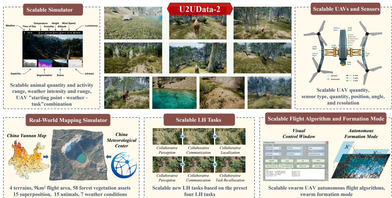
Figure 1: U2UData-2 collects a large-scale swarm UAV autonomous flight dataset for Long-Horizon (LH) tasks. U2UData-2 also provides a scalable data collection platform supporting the customization of simulators, UAVs, sensors, flight algorithms, formation modes, and LH tasks. Through its visual control window, U2UData-2 allows users to collect customized datasets through one-click deployment online and to verify algorithms by closed-loop simulation.
